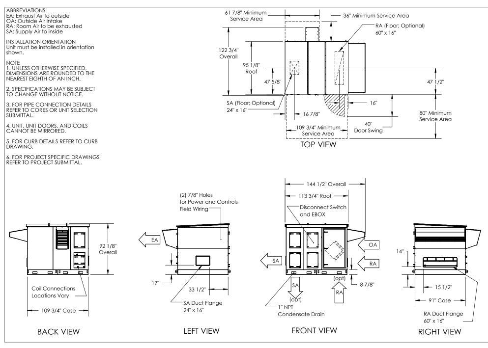
Model: DN-5JRT ERV+COIL 1" Drawing Type: Unit Dimension Version: DEC18
