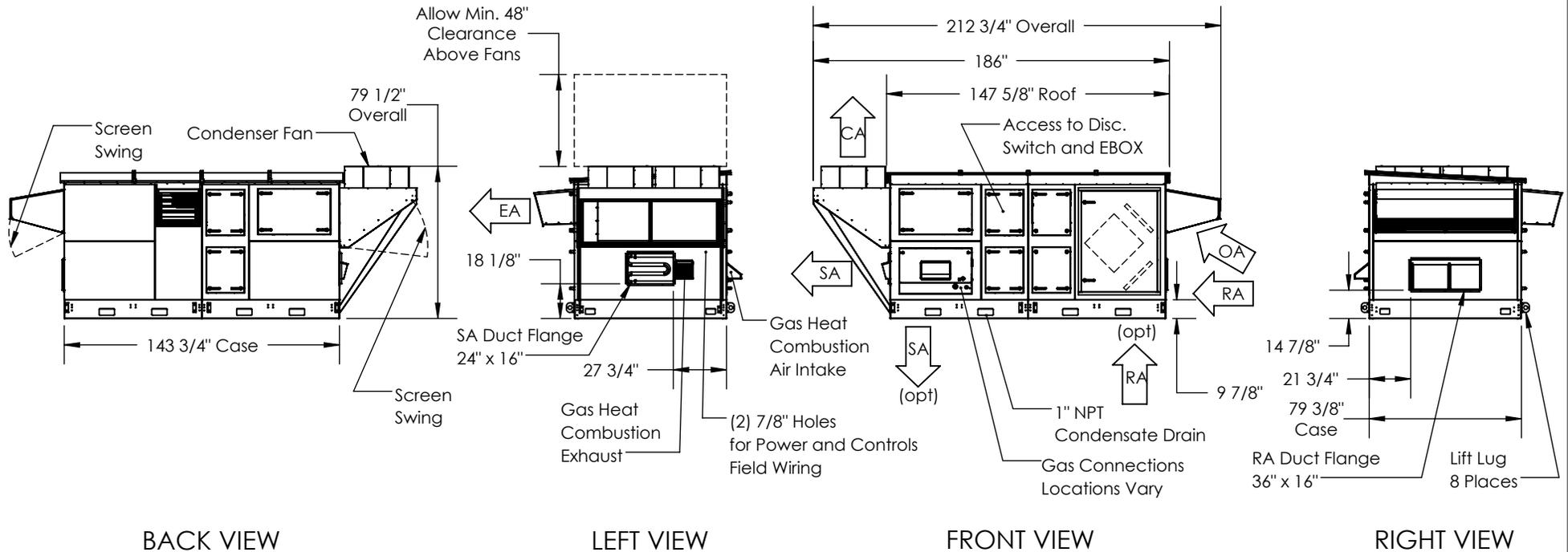
Model: DN-3JRT-PKGD ERV+COIL+HEAT 2"
