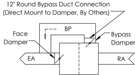
**BYPASS AIRFLOW SCHEMATIC
