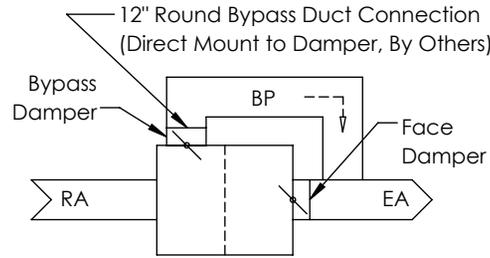
**BYPASS AIRFLOW SCHEMATIC
