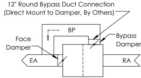
**BYPASS AIRFLOW SCHEMATIC**
