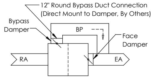
BYPASS AIRFLOW SCHEMATIC
