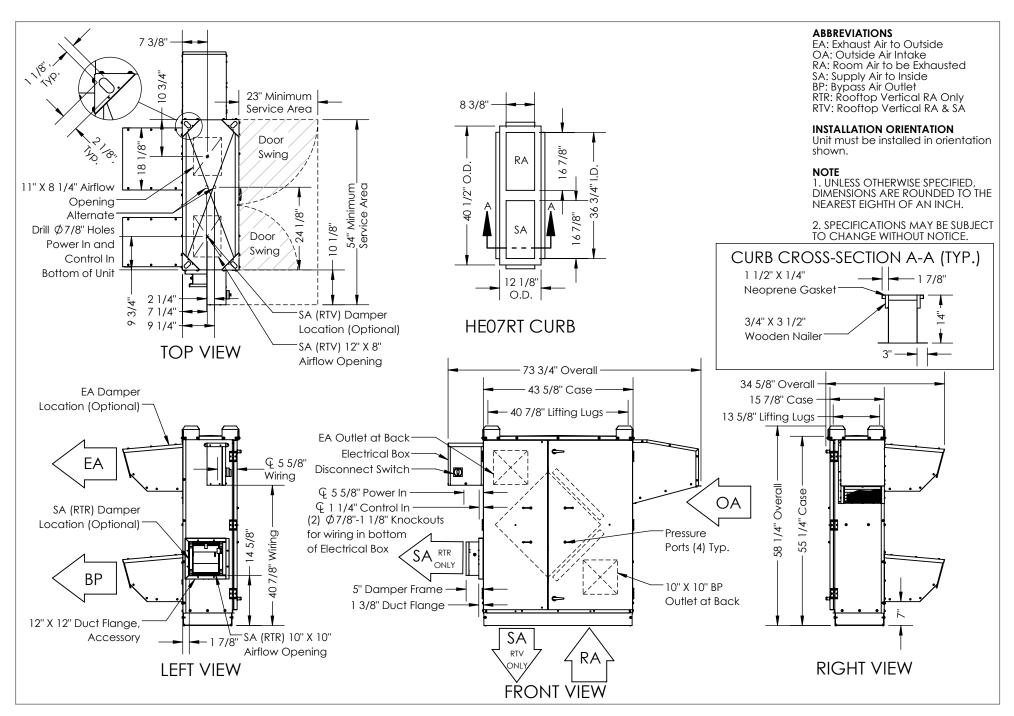
Model: HE07 RTR/RTV [Bypass] Drawing Type: Unit Dimension Version: JAN25
