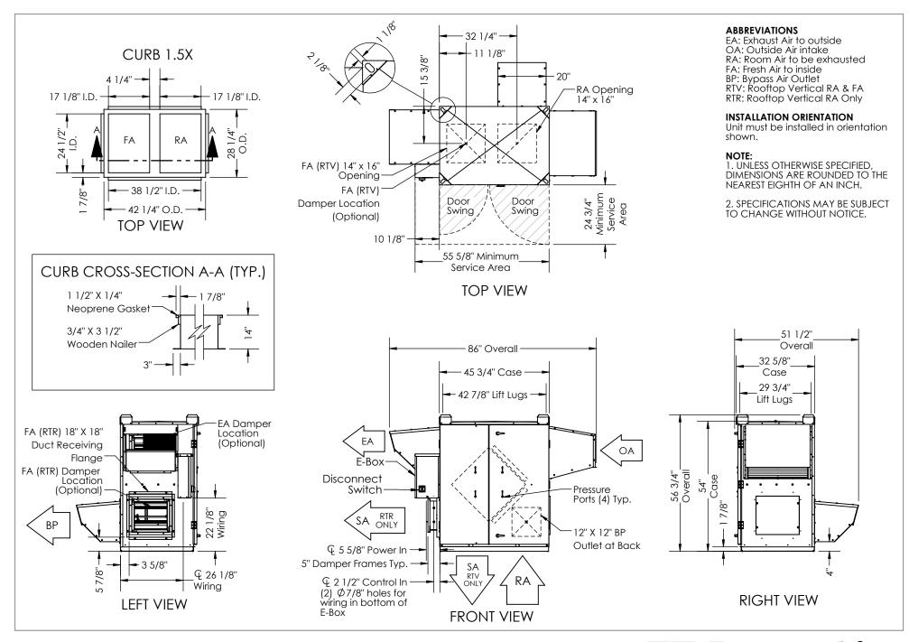
Model: HE1.5X RTV/RTR [BYPASS] Drawing Type: Unit Dimension Version: JAN25
